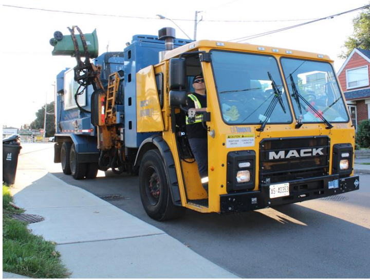
Figure 2: Side loader natural gas RCV (photo courtesy of City of Toronto Council, Canada)
