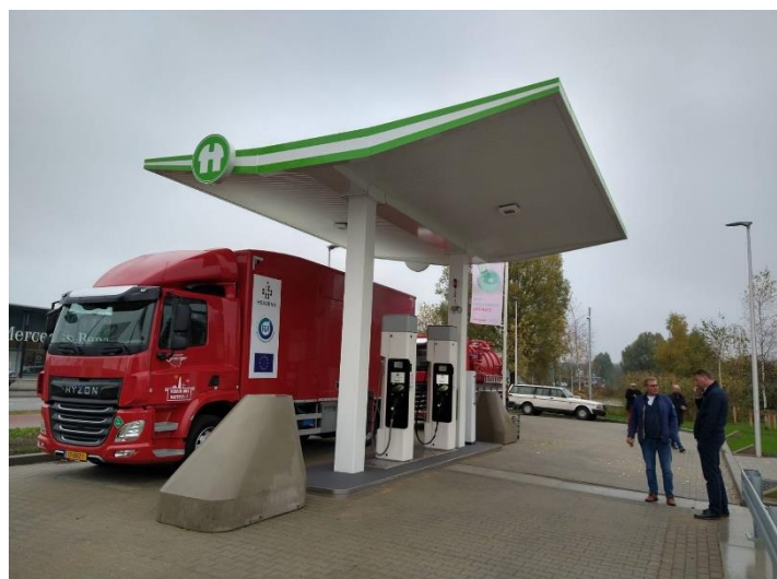
Figure 13: Hydrogen fuel cell RCV refuelling (photo courtesy of City of Groningen, Netherlands - photographer Martin Vonk)
