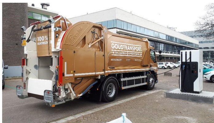
Figure 1: Electric RCV charging (photo courtesy of Rotterdam City Council, Netherlands)
